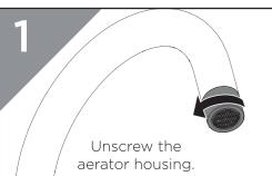
Remove the aerator from housing. Clean and replace as necessary.
