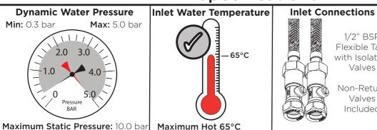
Flexible Tails with Isolation Valves Non-Return Valves
