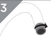
Secure the aerator. Turn on the mains water supply, letting the water flow for a few minutes to flush through the system.
