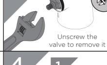
Reverse the steps to replace the valves and handles.
