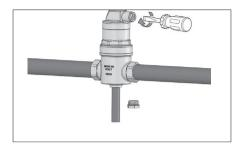
It is important to make sure that the air vent screw is always unscrewed to vent the air automatically.
