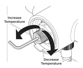
Wait for a couple of minutes for the temperature to stabilise after adjusting. Measure the water outlet temperature using a thermometer. Adjust until the desired temperature is reached.
