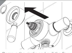
Remove the circlip and pull the flow handle off of the valve
