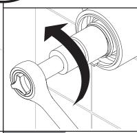
Use a 30mm socket spanner to unscrew the cartridge from the valve body. Carefully remove the cartridge and spring.
