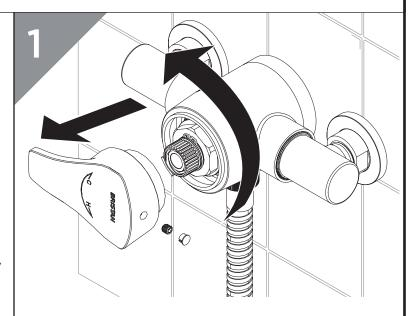
Turn the temperature handle to the maximum temperature. Undo the grub screw to remove the handle.
