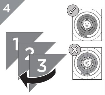
Reverse the steps to re-fit the cartridge and handle. Ensure the temperature stop is fitted correctly. The stop should sit at the bottom left, aligned centrally to the cartridge. Reset the maximum temperature.
