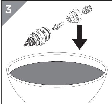
Remove all seals and check for any damage. Place the cartridge in a suitable solution and soak until fully de-scaled. Rinse thoroughly. Replace all seals and grease with a WRAS approved sealant.
