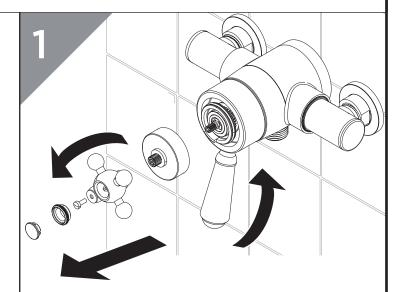
Turn the temperature handle to the maximum temperature. Remove the temperature handle and unscrew the shroud. Turn on the shower.
