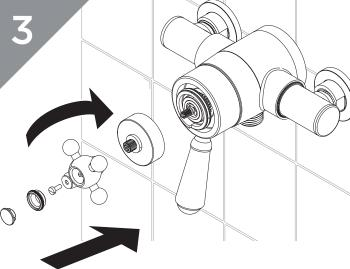
Re-fit the temperature handle back in the maximum temperature position.
