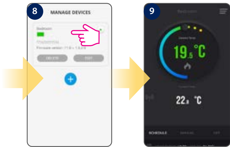
Tap anywhere on tile to enter the thermostat interface.
