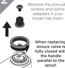
When replacing, ensure valve is fully closed with the handle parallel to the
