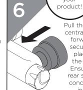
Pull the front 8 central shroud forward to secure into place on the valve. Ensure the rear shrouds conceal the
