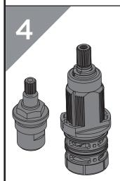
Remove O-rings and soak all components in de-scaler until fully de-scaled. Rinse thoroughly in clean water to remove all chemicals and debris.
