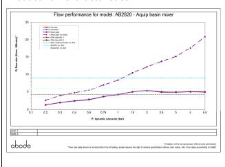
Min / Max water pressure (bar): 0.50\* / 5
