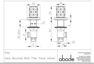
• Product mounted where: Surface • Recommended hole size:  $0 \, \text{mm}$
