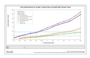
• Min / Max water pressure (bar): 1.40\* / 5
