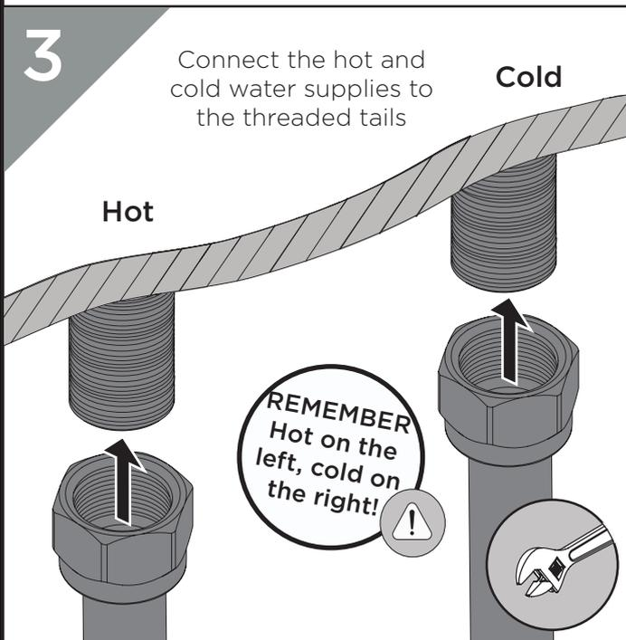
Connect the hot and cold water supplies to the threaded tails
