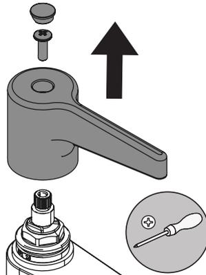
Unscrew handle and washer to remove the handles.
