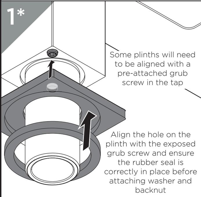
Some plinths will need to be aligned with a pre-attached grub screw in the tap
