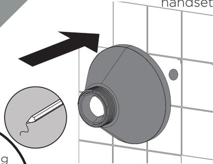
On most models, the screw holes are large enough to fit a pencil through for easy marking.
