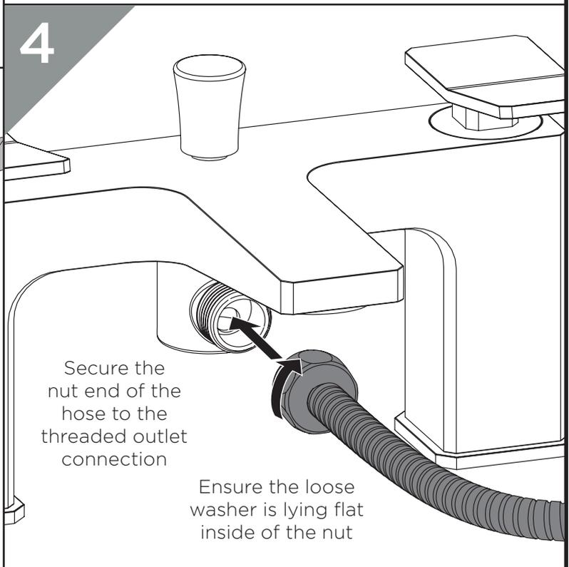
Secure the nut end of the hose to the threaded outlet connection
