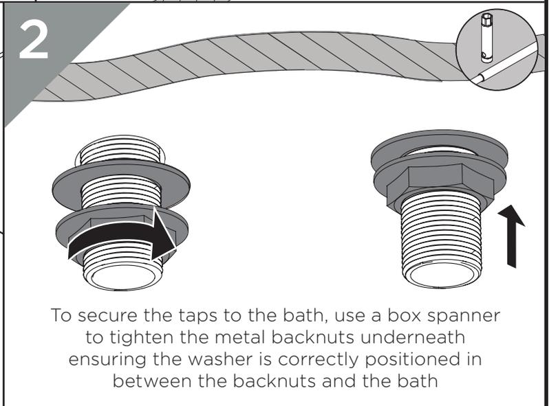
To secure the taps to the bath, use a box spanner to tighten the metal backnuts underneath ensuring the washer is correctly positioned in between the backnuts and the bath
